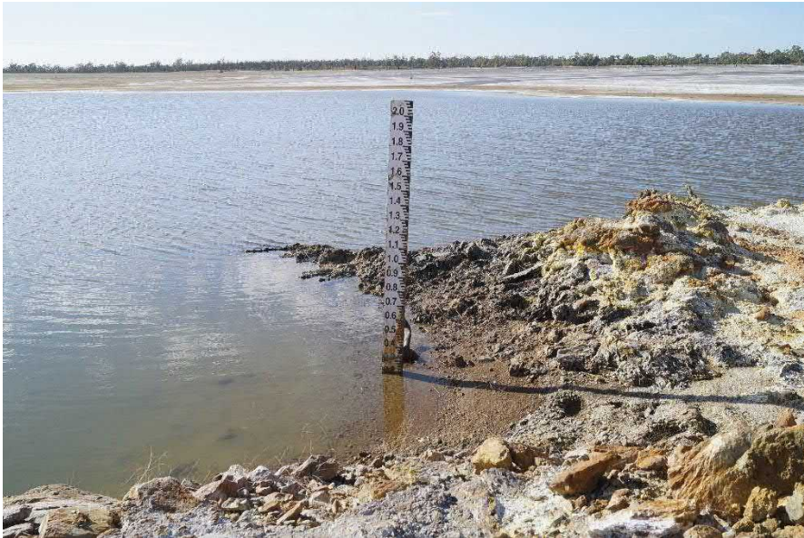
Water level measuring staff (17/2/2022)
