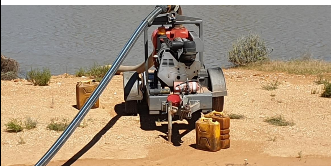
Photo 6: Fuel tanks kept without bunding (NC 19)
