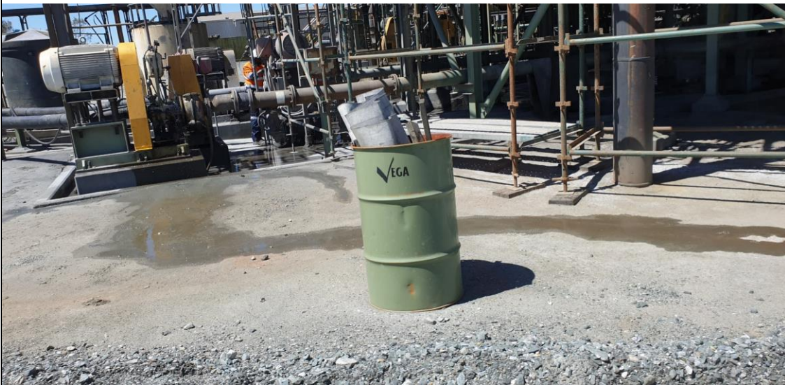
Photo 7: Random placement of unlabelled containers around plant area (NC 19)
