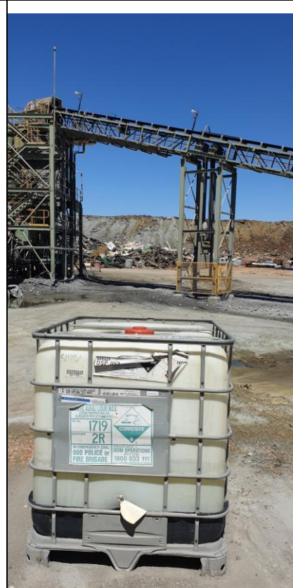
Photo 3: Some IBCs are randomly placed around the site without bunding (NC20)
