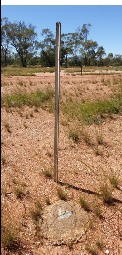
Photo 1: Survey Mark maintained and protected
