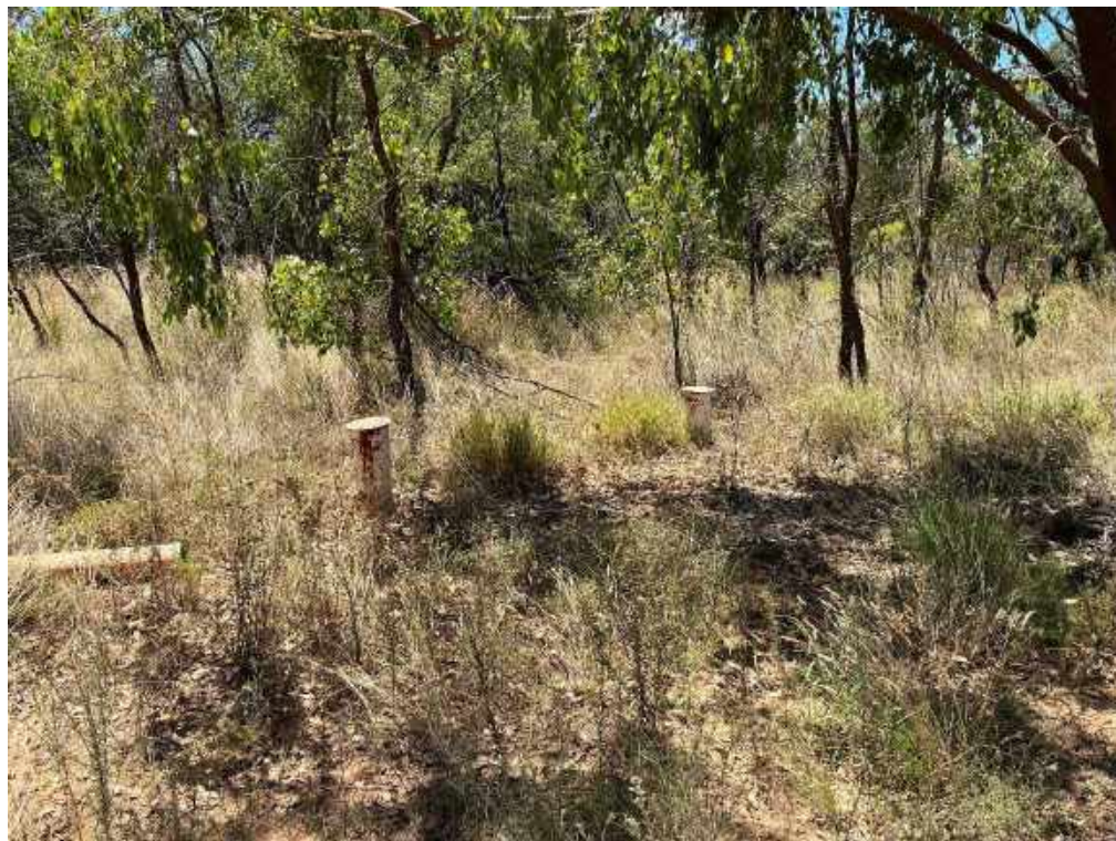
PZH002D and S suite of bores downstream of main embankment.
