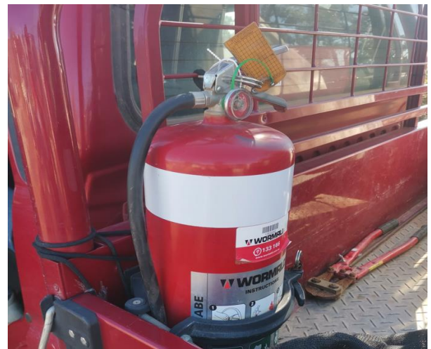
Photo 6 Fire extinguisher in rear of site vehicle
