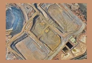
Great progress is underway on the Heap Leach Cells as part of our site rehabilitation efforts. We're carefully and safely layering rock over the cells and the valleys between them to create the final landform. Each layer of the cover is tested to ensure proper drainage and compliance with rehabilitation standards.
