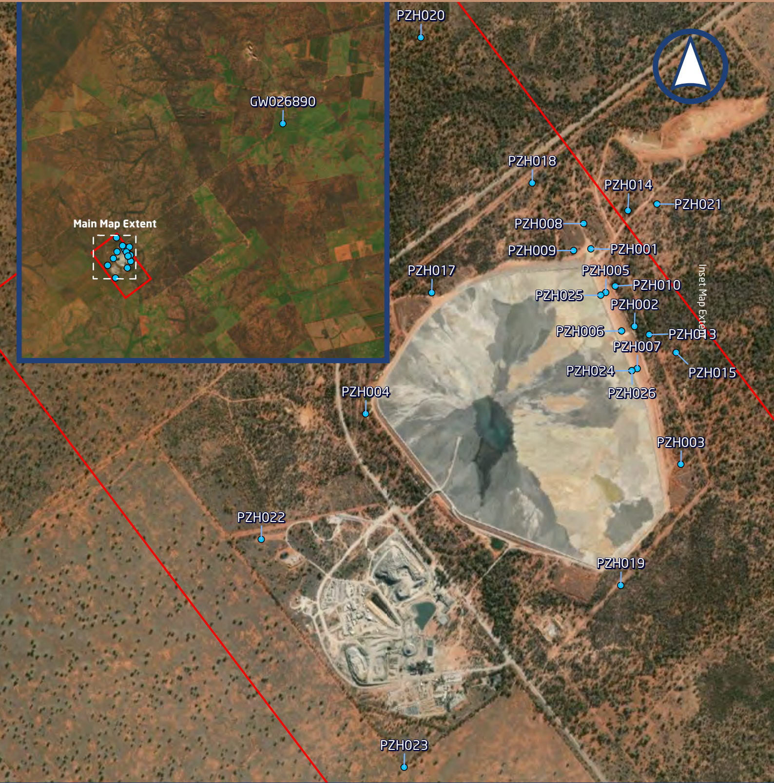
Figure 8 - Groundwater Monitoring Locations
