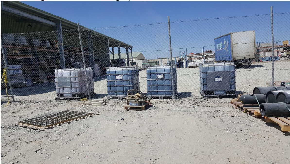
Storage of IBCs without bunding
